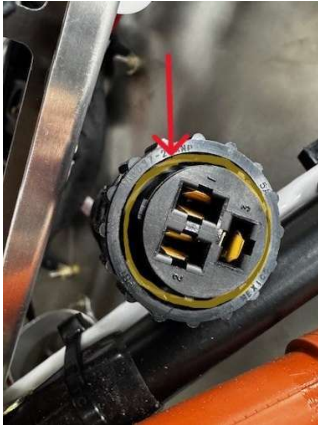
Figure 2. Male side fusebox connector. (Rubber seal location highlighted in yellow for clarity)
