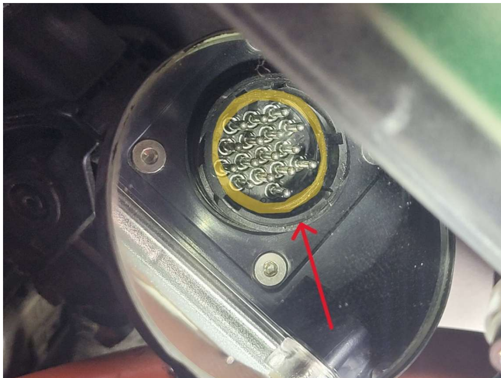
Figure 3. Fusebox connector with seal. (Rubber seal location highlighted in yellow for clarity)
