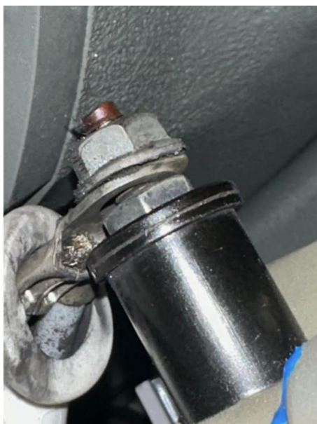
Figure 4: Examples of visible play on stud and thermal/corrosion damaged hardware
