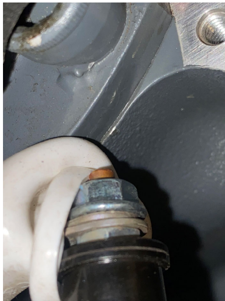
Figure 3: Example of incorrect hardware that is tight and undamaged
