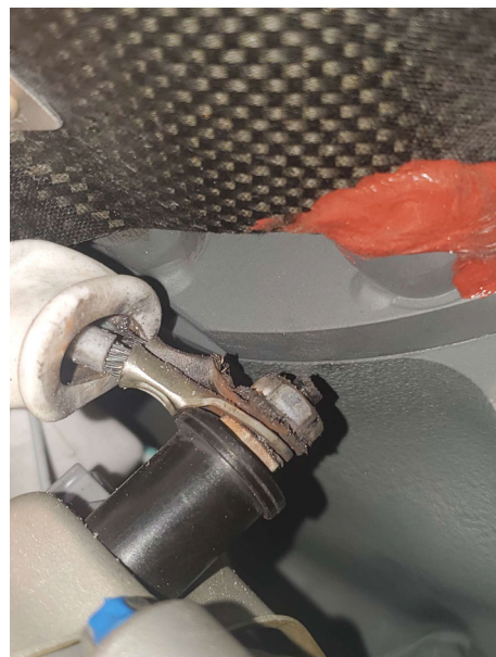
Figure 4: Examples of visible play on stud and thermal/corrosion damaged hardware
