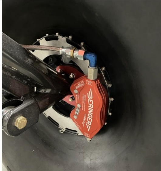
Figure 16 - Completed brake installation
