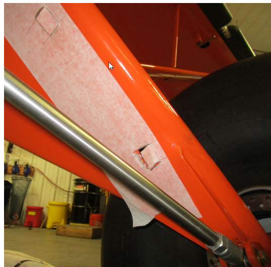
Figure 7 – Access flaps in fabric
