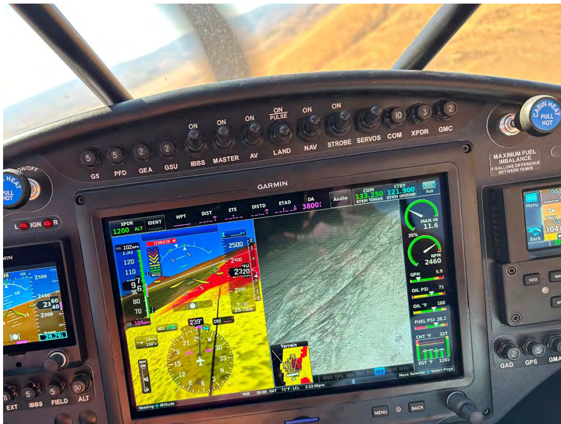
A CubCrafters Carbon Cub with a G3X integrated thermal infrared camera system avoids terrain during company camera testing near Yakima, WA – Photo courtesy of CubCrafters
