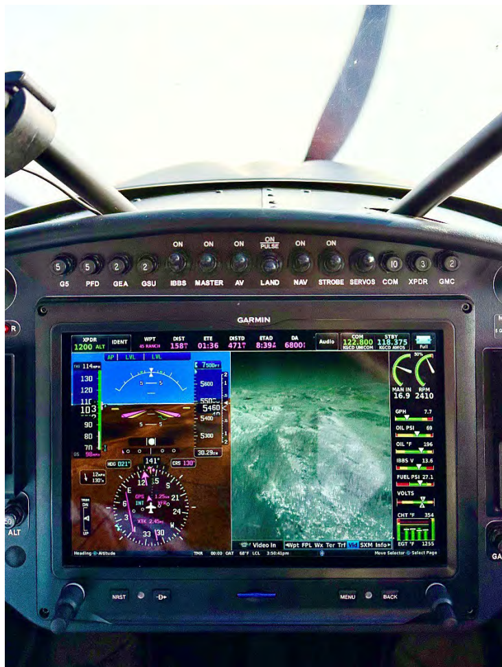
IR camera performance with less than ½ mile forward visibility in forest fire smoke. – Photo courtesy of CubCrafters
