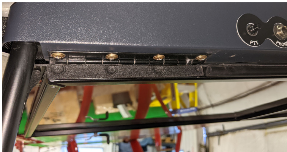
FIGURE 5 – Foam Seal on Window Hinges
