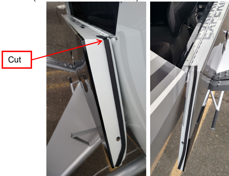
FIGURE 1 – Foam Seal on Door
