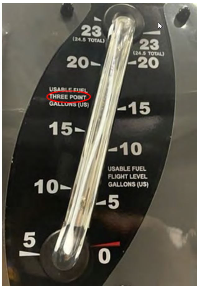
Figure 33 – Incorrect Placard (replace)
