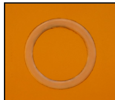
FIGURE 3 –Grommet installed on Wing Exterior
