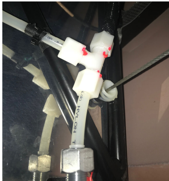
Figure 5 - Nylon Union Tee Fuel Fitting, Aft Right
