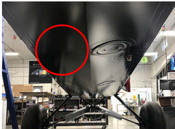
Figure 6 - New Inspection Panel Location
