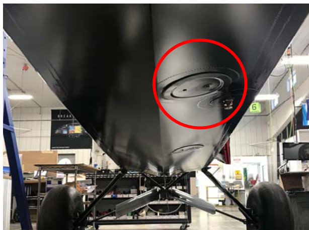
Figure 3 - Inspection Panel Location, Extended Baggage
