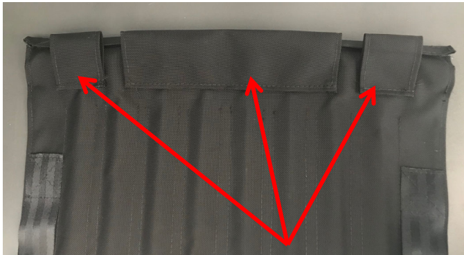
FIGURE 2 – Aft Sling Seat Seam, Bottom View
