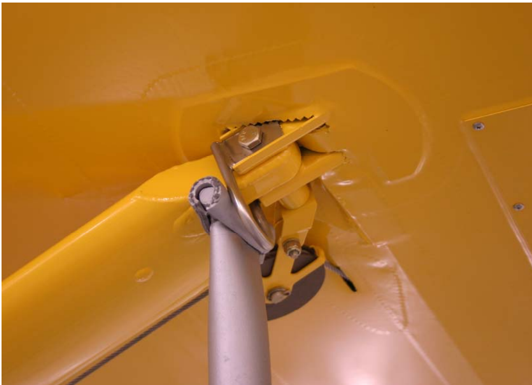
FIGURE 07-00-3 - Jacking From the Wing
