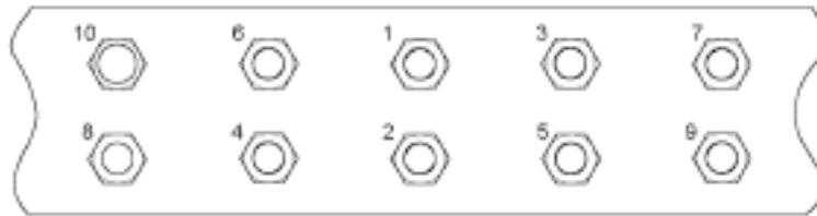
TYPICAL LINEAR PATTERN TORQUING SEQUENCE
