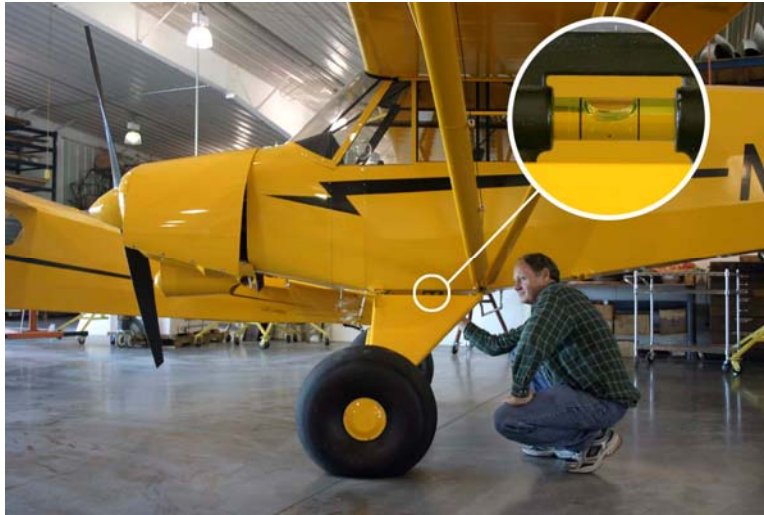
Figure 08-00-1 - Leveling the Aircraft Longitudinally
