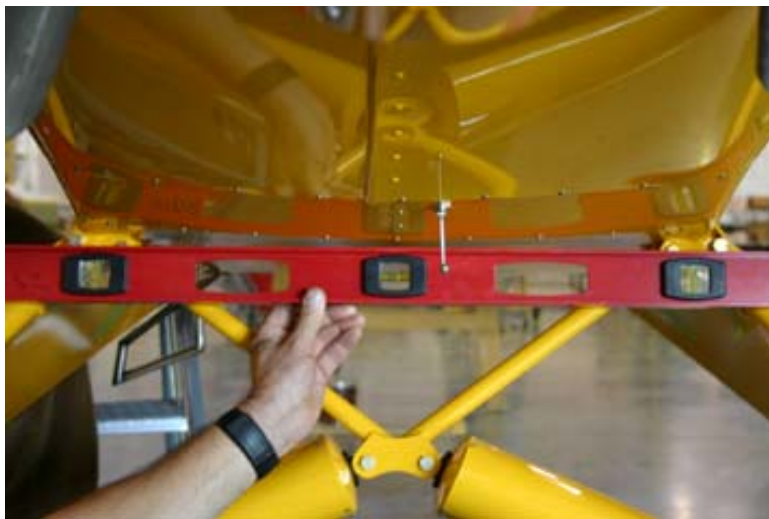
Figure 08-00-2 - Leveling the Aircraft Laterally
