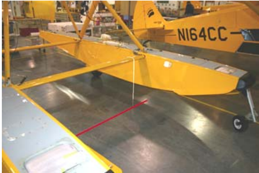
Figure 08-00-8 Measuring the Arm on Aircraft Equipped with Wipaire 2100A Amphibious Floats
