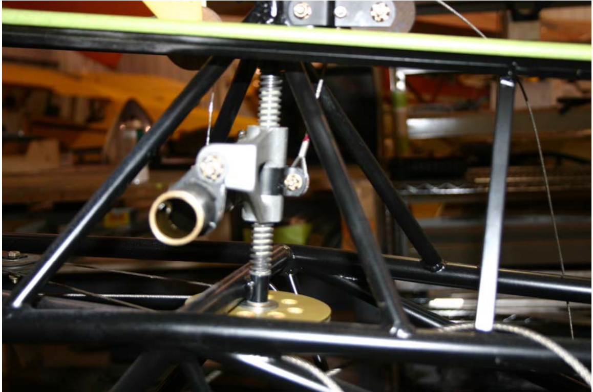
Figure 27-40-5 - Yoke in the Center of the Jackscrew
