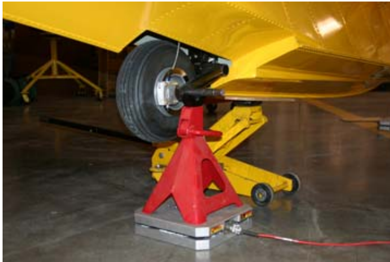
FIGURE 08-00-3 - Jacking Aircraft with Wipaire 2100A Amphibious Floats
