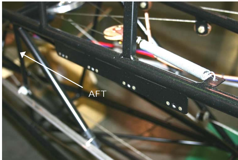
Figure 27-40-8 - Bracket for Strake Attachment – RH Shown
