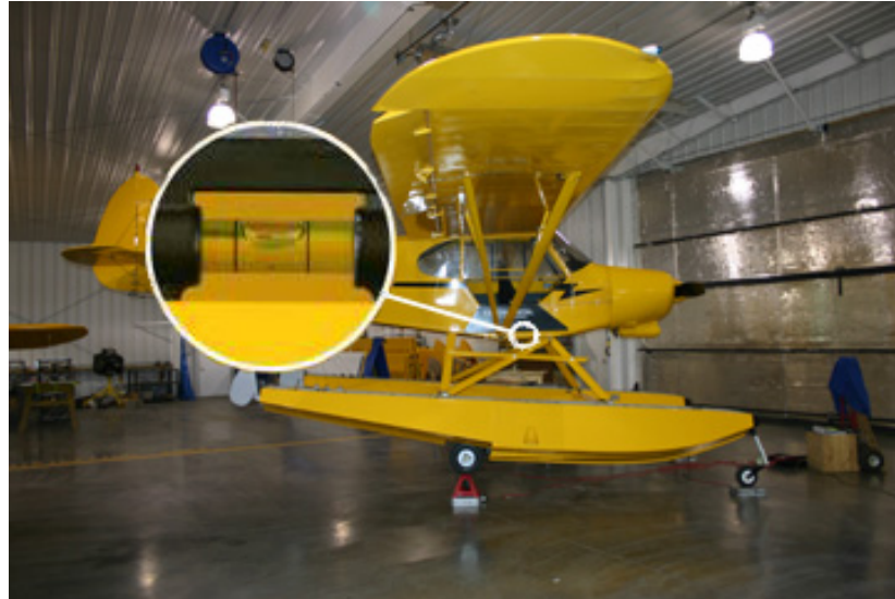
FIGURE 08-00-4 Leveling Aircraft with Wipaire 2100A Amphibious Floats Longitudinally
