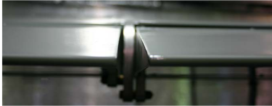
Figure 6.3.6.4: Alignment of Aileron Trailing Edge with Flap Trailing Edge
