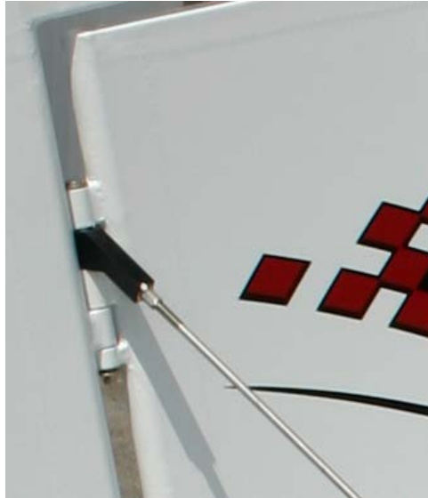
Figure 6.3.5.2: Installation of Clevis Pins at Rudder Hinges
