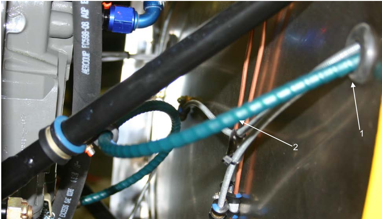
1 - Firewall 2 - Throttle Cable
