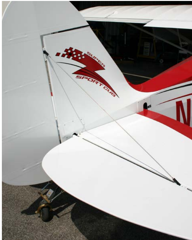
Figure 6.3.5.5: Tail Brace Wires and Elevator Attachment
