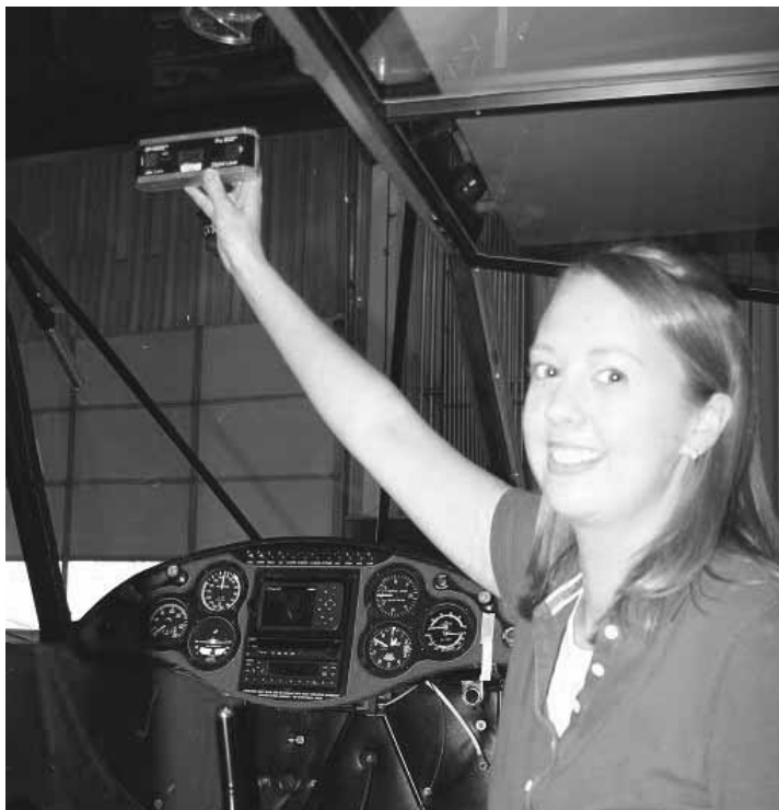
Figure 6.3.22.2: Leveling the Aircraft Laterally
