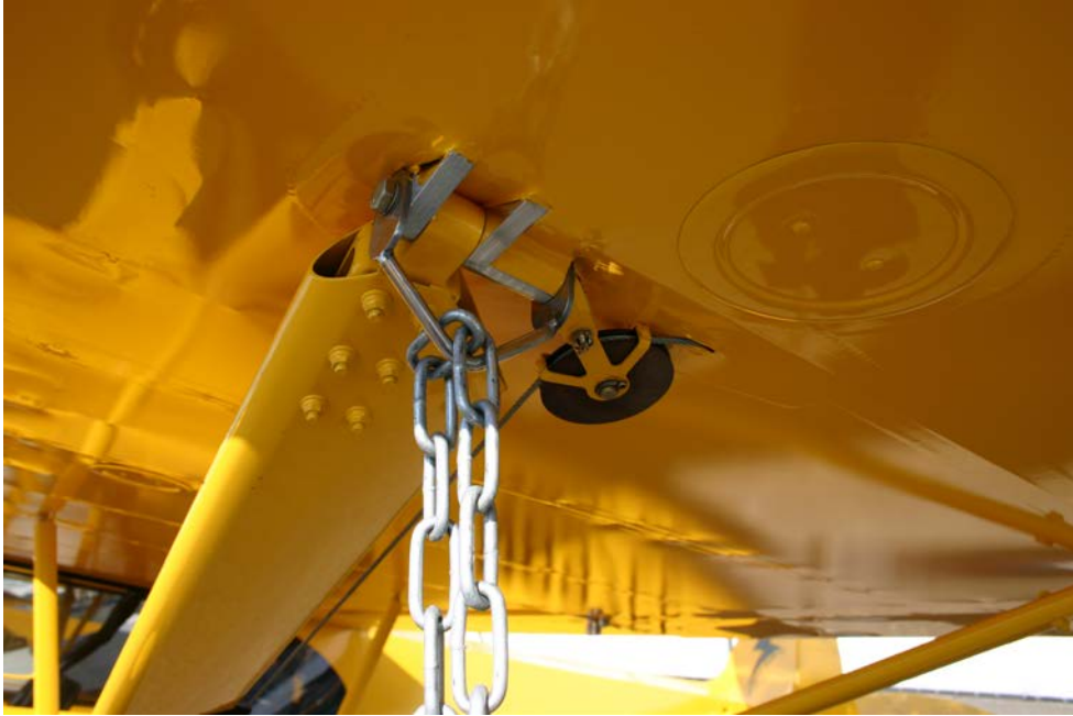
Figure 6.3.24.1: Wing Tie Down
