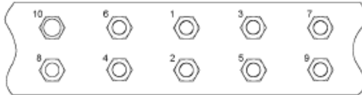
TYPICAL LINEAR PATTERN TORQUING SEQUENCE
