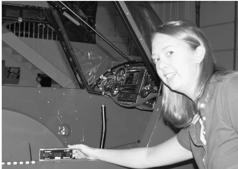
Figure 6.3.22.1: Leveling the Aircraft Longitudinally
