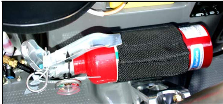
FIGURE 2 – Correct Fire Extinguisher Installation
