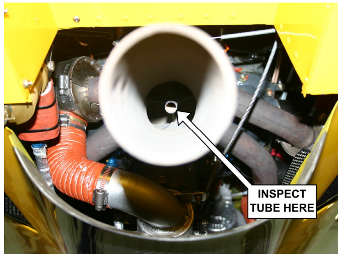
Figure 1 – Oil Breather Tube in Exhaust: View Looking Forward
