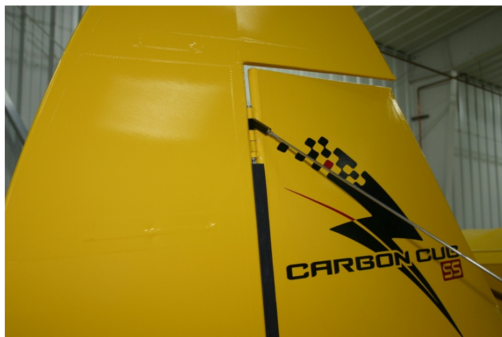
FIGURE 3 - Installing Rudder Gap Seal
