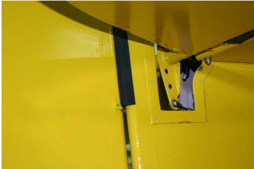
FIGURE 5 – Lower Rudder Gap Seal Position with Navigation Light Wire
