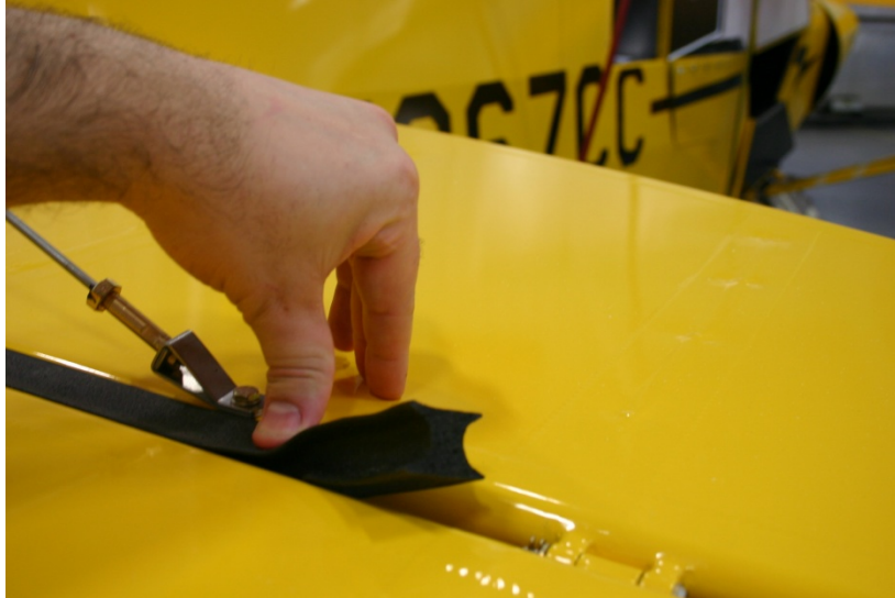
FIGURE 1 - Installing Elevator Gap Seal Between the Hinges
