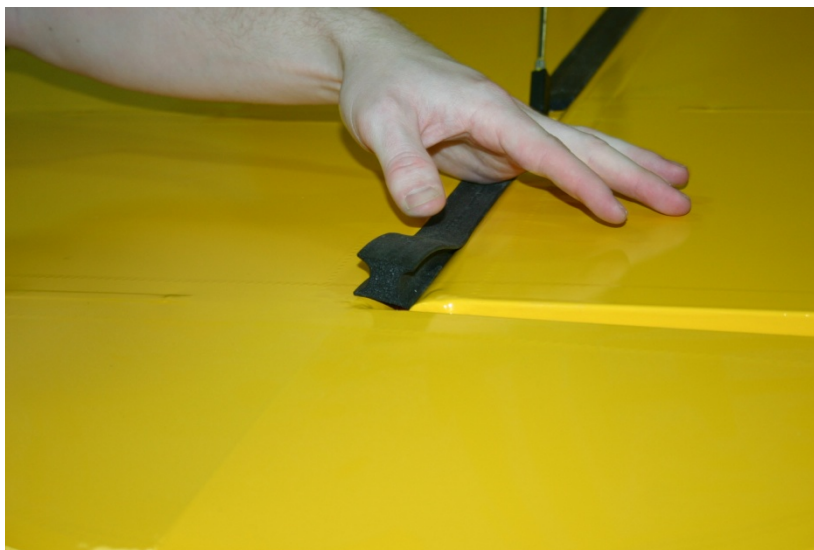
FIGURE 2 - Installing Elevator Gap Seal Between the Outboard Hinge and the Horn
