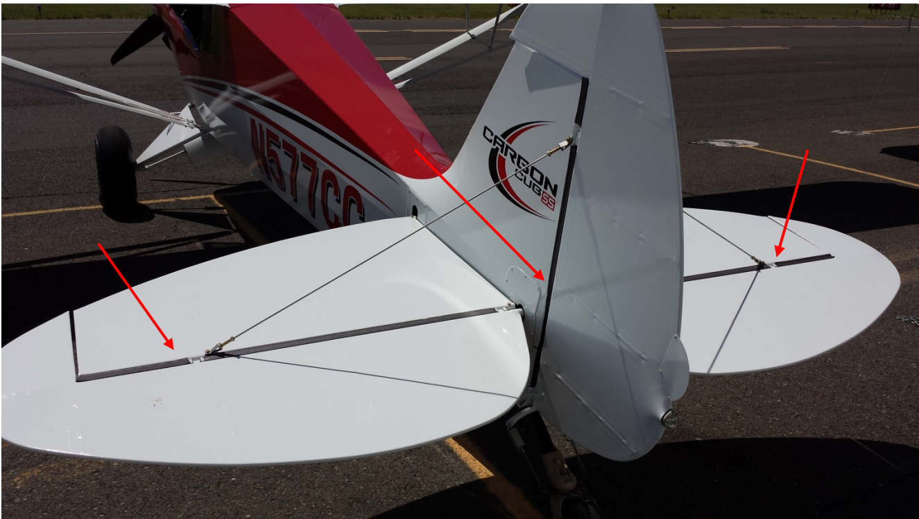
FIGURE 6 – Gap Seals Installed
