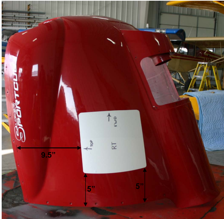
FIGURE 1 - CC11-160 Cowl Flap Retrofit Template Location
