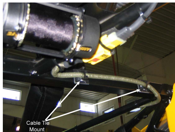
FIGURE 2 – Cable Tie Mount Installation
