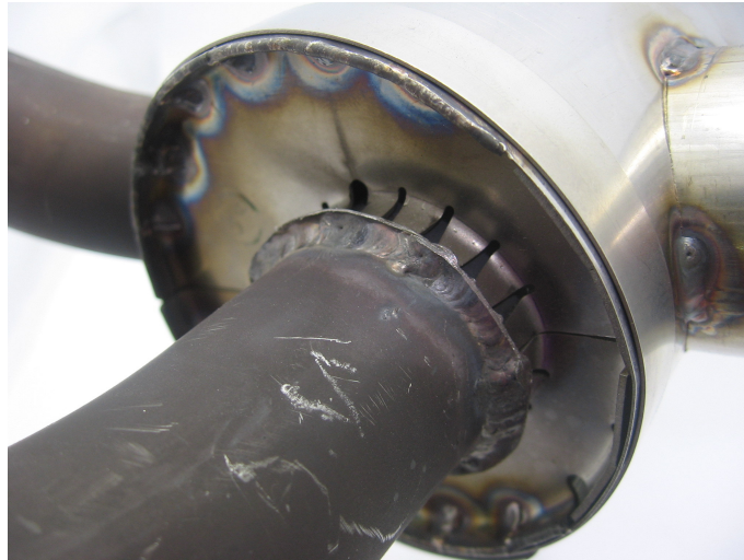
FIGURE 1: Remove Bulkhead and Install New Muffler Assembly
