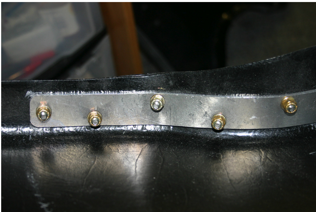
FIGURE 10 –COMPLETED INSTALLATION ON SEAT BACK
