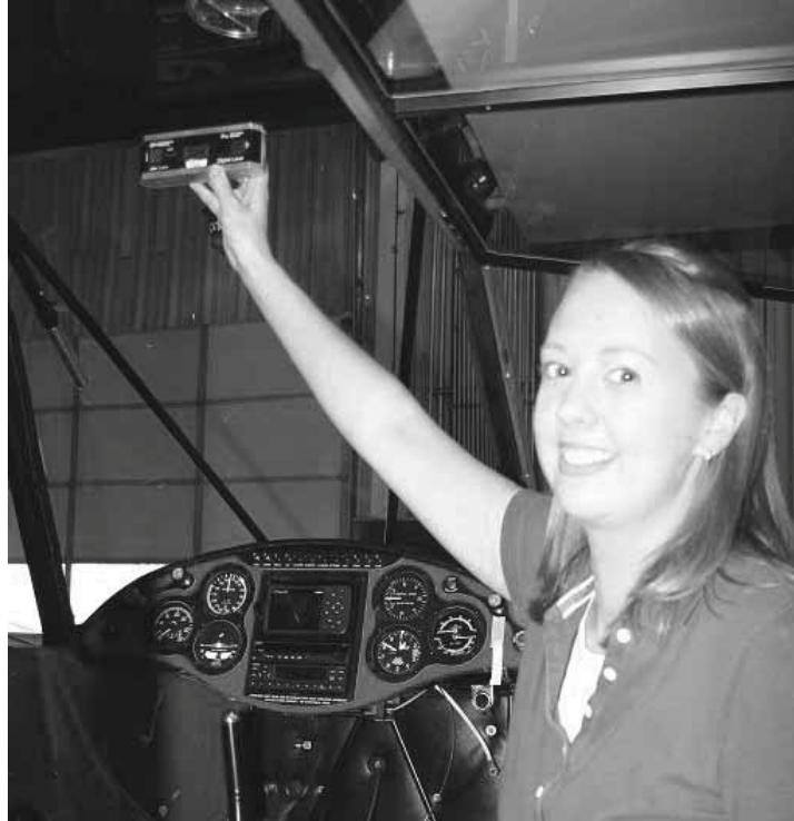
Figure 6.3.22.2: Leveling the Aircraft Laterally
