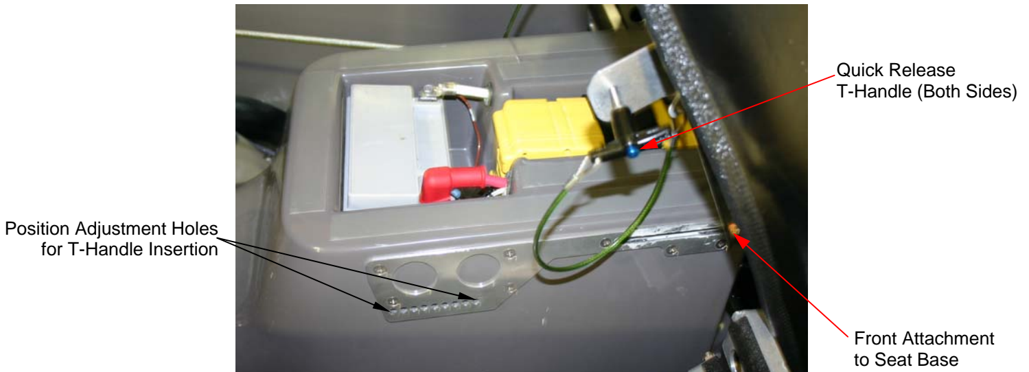
Figure 1 - Front Seat Attachment
