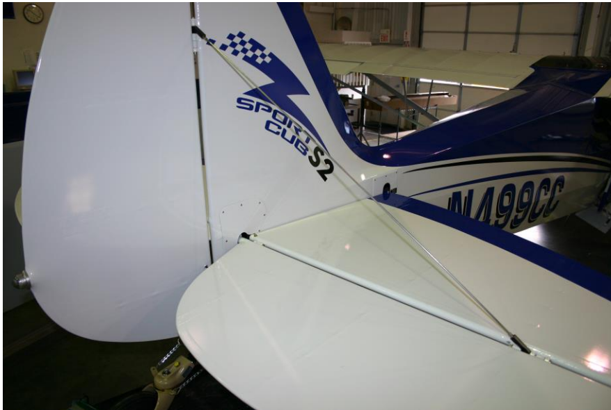
Figure 6.3.5.5 Tail Brace Wires and Elevator Attachment
