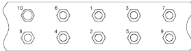
TYPICAL LINEAR PATTERN TORQUING SEQUENCE
