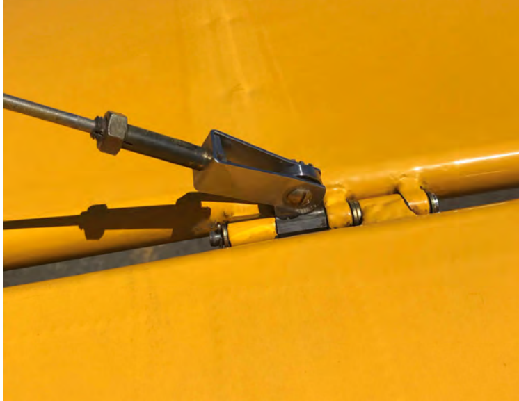
Figure 6.3.5.8 Clevis Pin Installation on Elevator
