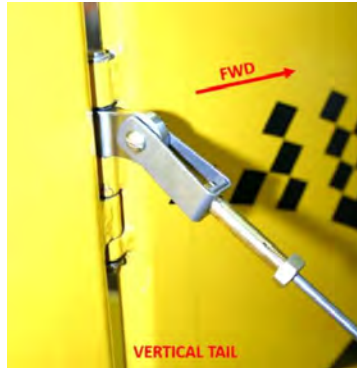
Figure 6.3.5.2 Installation of Clevis Pins at Rudder Hinges
