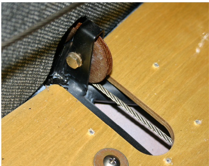
FIGURE 2 – Cover Removed-Inspection of Pulley Diameter
