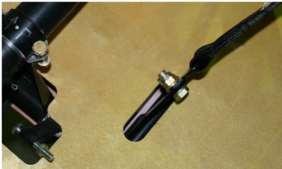
FIGURE 1 –Pilot Right Side Lap Belt Attachment, Lock Nut (Head of Bolt Facing Aircraft Centerline)
