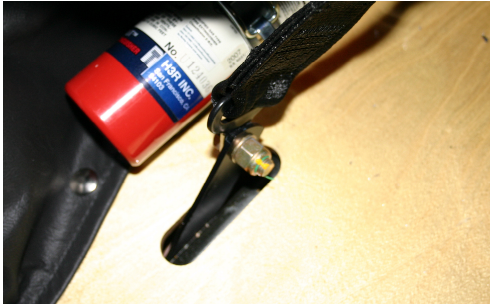
FIGURE 1 –Pilot Right Side Lap Belt Attachment, Lock Nut (Head of Bolt Facing Aircraft Centerline)
