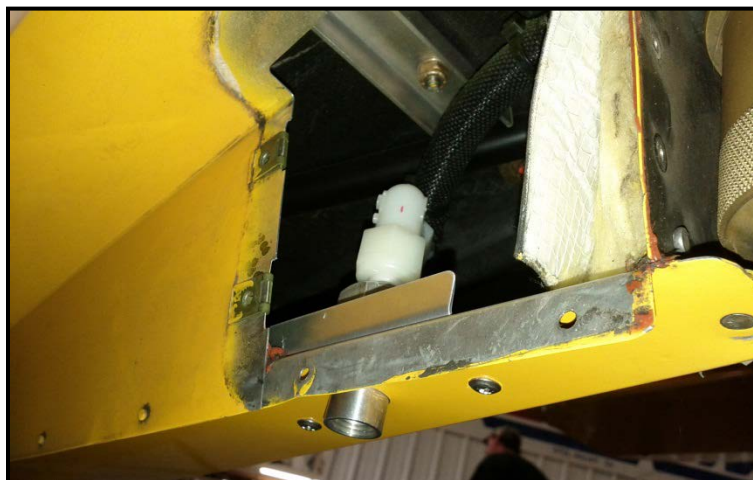
FIGURE 23 – Truss Head Screws as Installed
