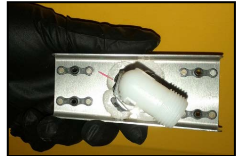
FIGURE 21 – Elbow Orientation (Note the parts flare aft)
