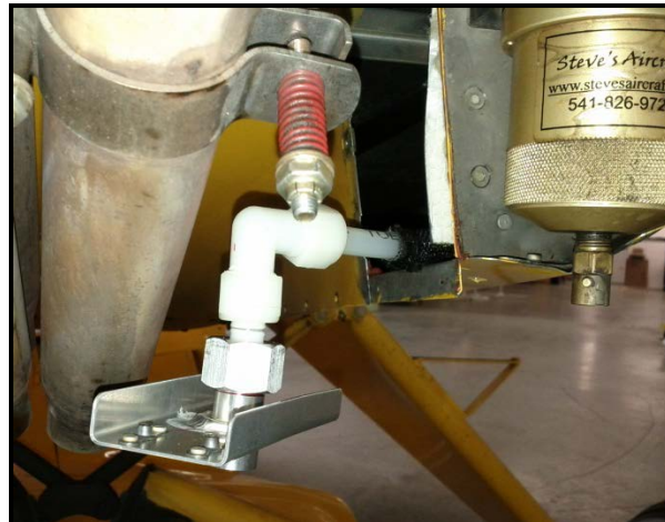
FIGURE 22 – Elbow Assembly as Installed
