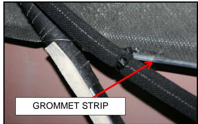
FIGURE 9 –Composite with Grommet Strip Installed
