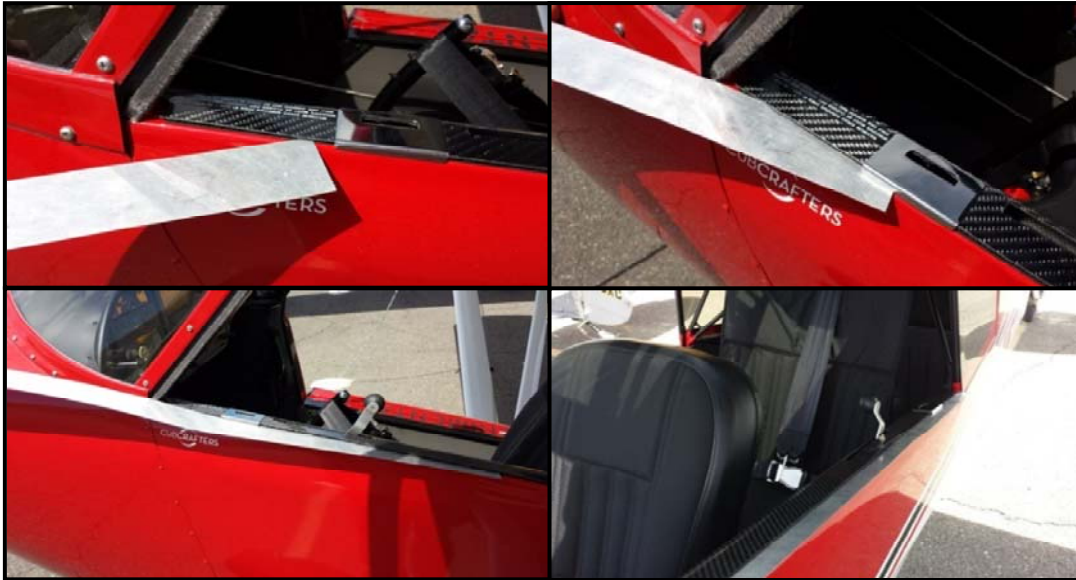
FIGURE 2 - Metal Strap Placement
