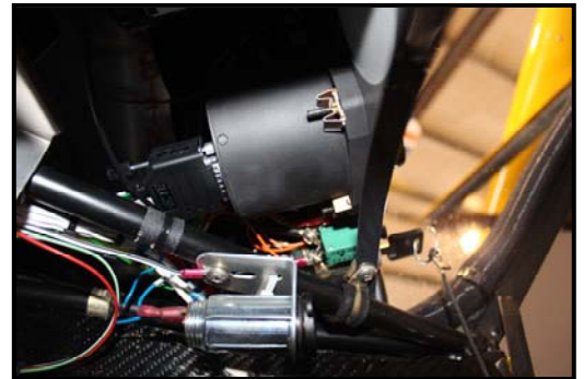
FIGURE 11 – Electronic Gauge as Installed
