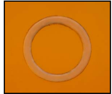
FIGURE 3 –Grommet installed on Wing Exterior
