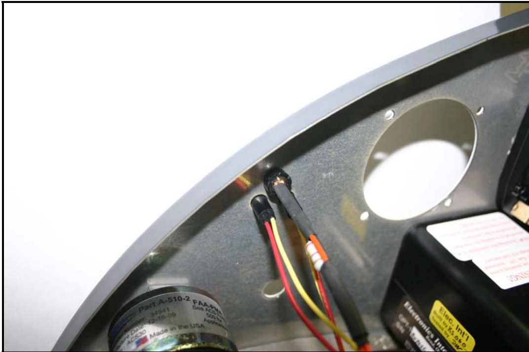
FIGURE 4 - Outer Ring snapped in Place
