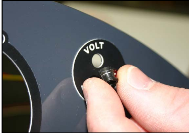
FIGURE 2 - Inner Ring Installation
