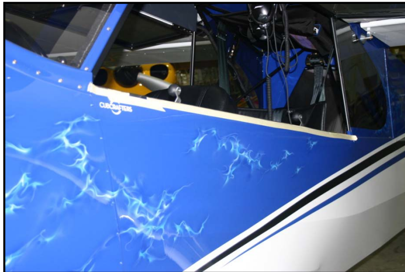
Figure 1 - Tape Installation on Fuselage
