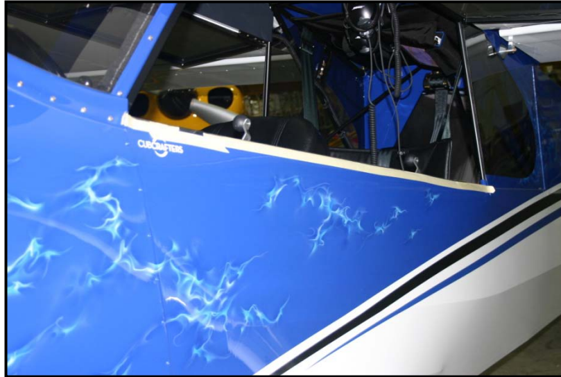
Figure 8 - Fuselage Tape Installation
