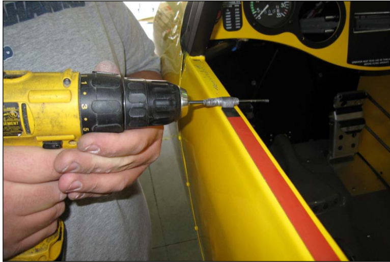
Figure 7 - Tape Removal from Fuselage
