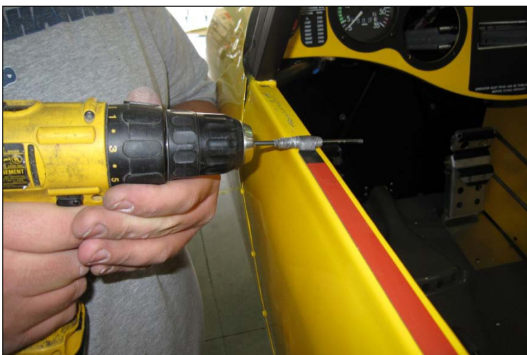
Figure 16 - Tape Removal from Fuselage
