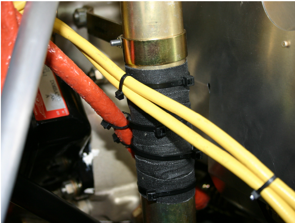
Figure 1 - Securing of the Oil Line to the Oil Filler Neck
