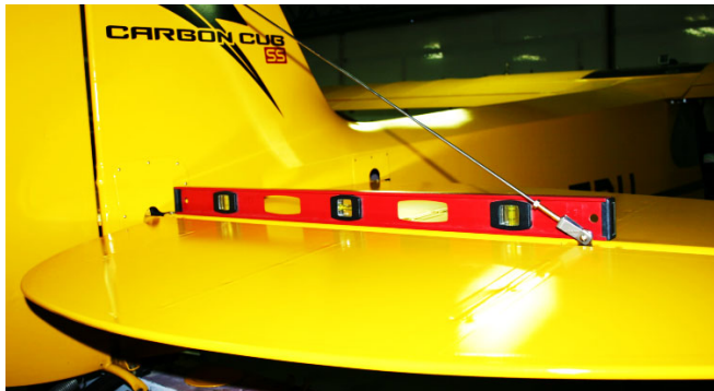
Figure 10: Leveling Horizontal Tail
