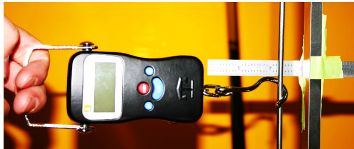
Figure 12: Wire Tension Measurement
