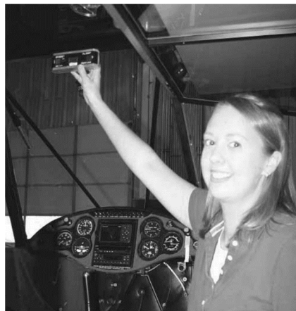
Figure 9: Leveling the Aircraft
