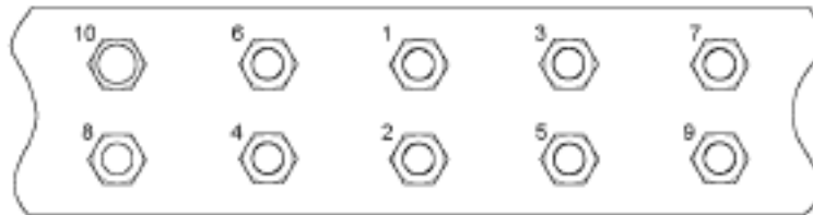
TYPICAL LINEAR PATTERN TORQUING SEQUENCE
