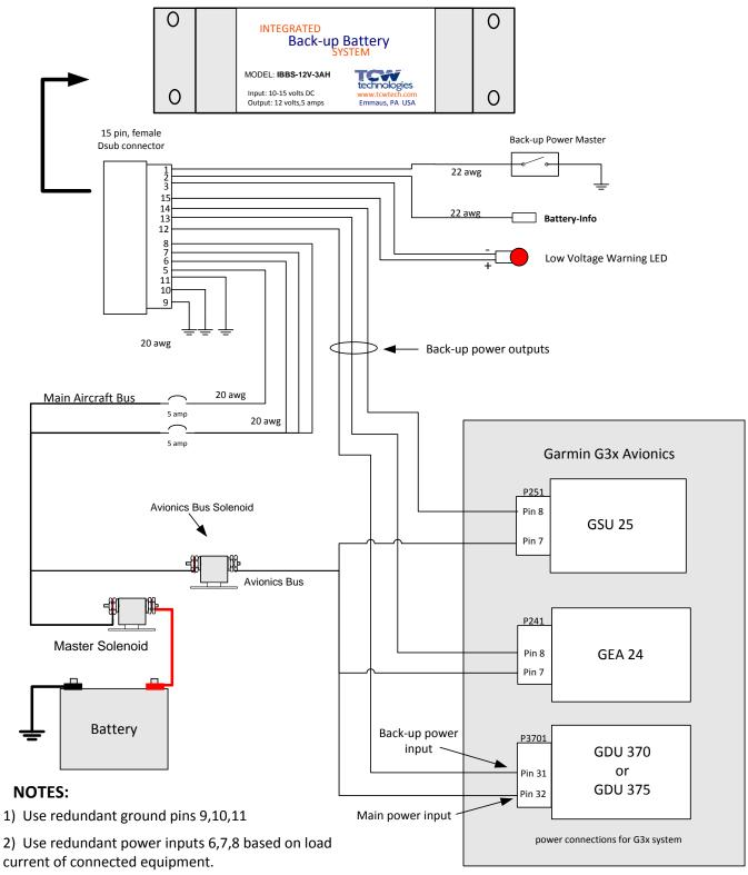
3) Use of pins 6,7,8 will power connected equipment even when avionics bus is OFF via pass thru mode. Use of input pins 6,7,8 is OPTIONAL.
