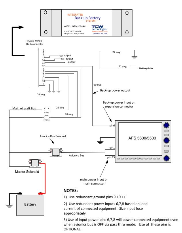
4) No back-up master switch required when wired per this drawing for AFS
