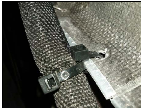
FIGURE 32 – Secure Round-It Protective Wrap using Cable Tie Chain
