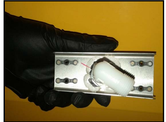
FIGURE 19 – Elbow Orientation (Note the parts flare aft)
