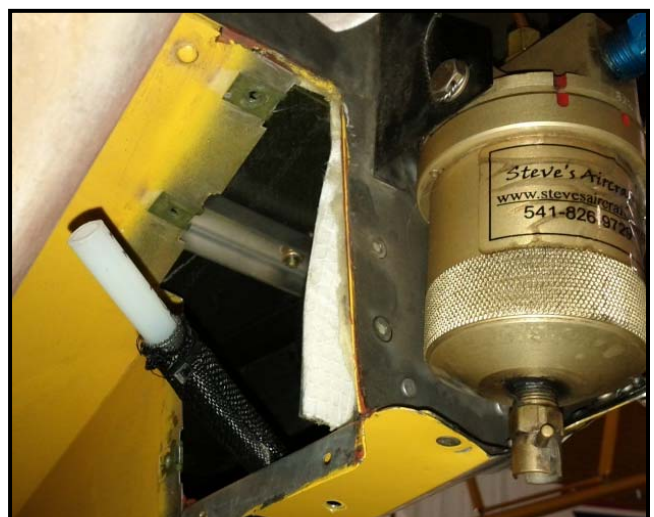
FIGURE 18 – Access Panel at Boot Cowl Showing Fuel Line Routing
