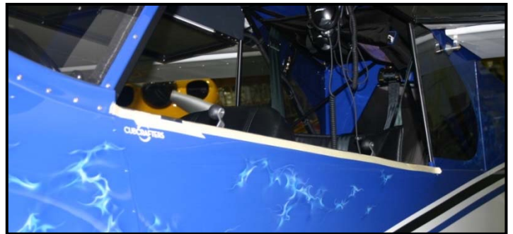
FIGURE 1 - Tape Installation on Fuselage
