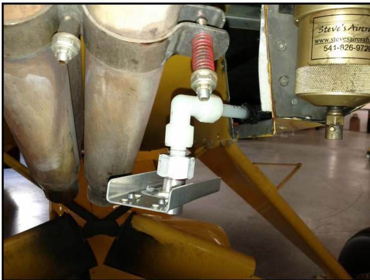
FIGURE 20 – Elbow Assembly as Installed
