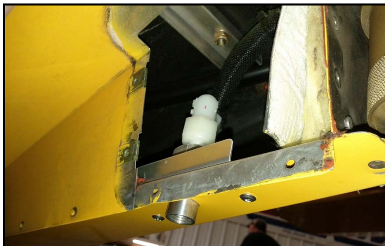
FIGURE 21 – Truss Head Screws as Installed
