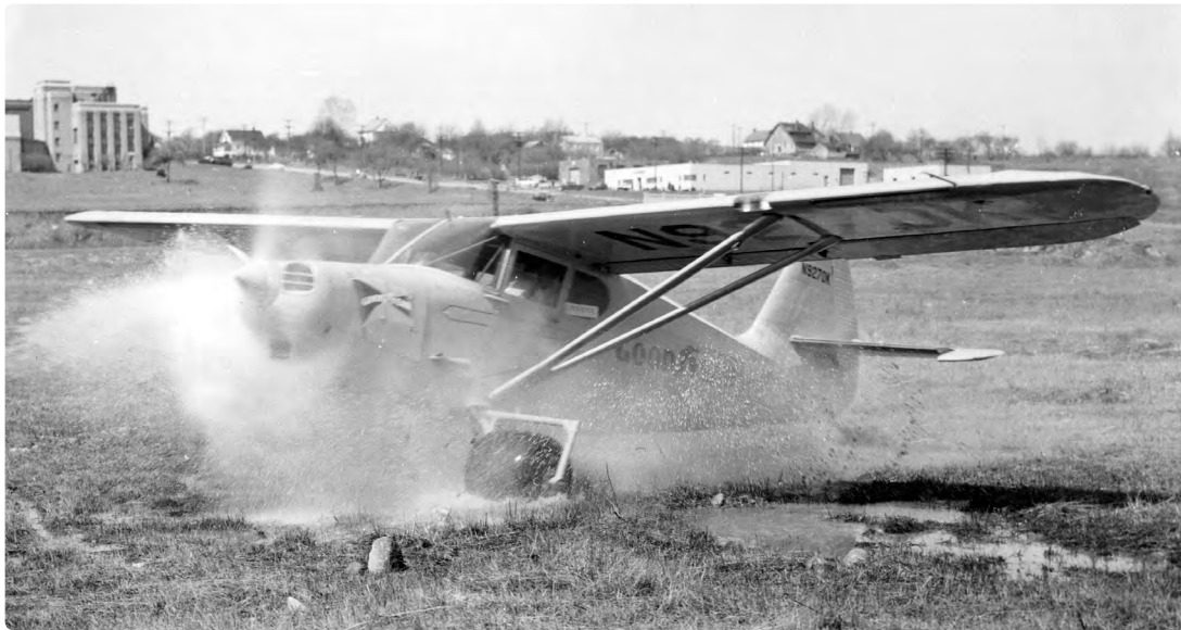
ABOVE The Stinson uses the 24in (61cm)-wide footprint of its Terra-Tires to roll across a field full of puddles and ditches with ease during trials. A large variant of the tyre was developed for use on the MM-1 Teracruzer missile-carrying vehicle built by the Four Wheel Drive Auto Company to transport the USAF's Martin MGM-13 missiles.
