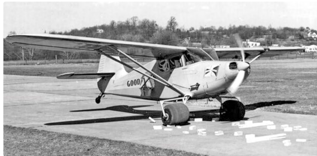
ABOVE The Voyager demonstrates its ability to deal with uneven surfaces on an obstacle course made of wooden blocks and planks during trials at Akron Fulton Airport (now Akron Executive Airport), which was opened in 1929 as the Goodyear Airdock, where the company's airships were built, and which also served as the Navy's NAS Akron.
